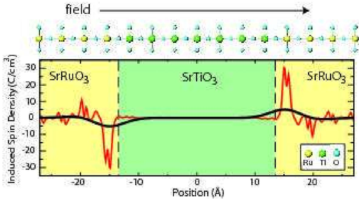
FIG. 1: (color online) Calculated magnetization induced by an external voltage of 27.8 mV in a nanocapacitor consisting of 7 layers of SrTiO<sub>3</sub> alternating with 7 layers of ferromagnetic, metallic SrRuO<sub>3</sub>. The light (red) and bold (black) lines show respectively the planar averaged, and macroscopically and planar averaged induced magnetization profiles.
